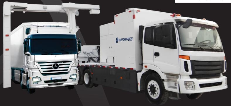
The HXM-MobileScan™ is a mobile cargo scanner designed for screening fully-loaded trucks, shipping containers, and delivery vehicles. Its high-powered generator provides 320 mm of steel penetration and allows operators to quickly check and verify shipping manifests. Wireless integrated networking capabilities enable it to share and transmit images, and its automated deployment system is simple to operate.
