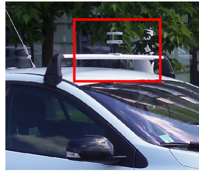
Fig. 3. The Velodyne VLP-16 is installed on the Renault Fluence ZE’s roof surface.
