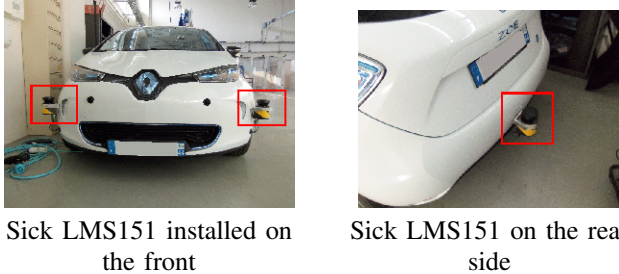
Fig. 2. The LiDARs Sick LMS151 are installed in strategical positions to ensure a 360°FoV around the vehicle.
