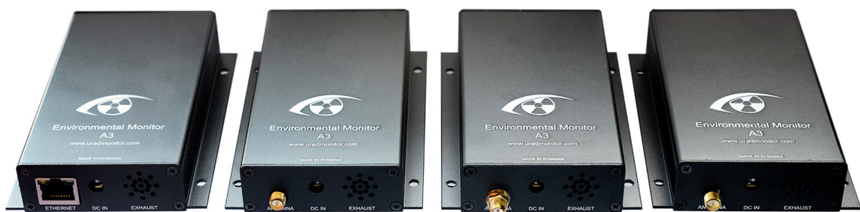
Ethernet, Wifi, GSM and LORAWAN
