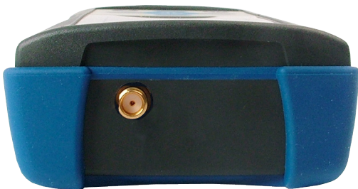
SNYPER Antenna Connector
