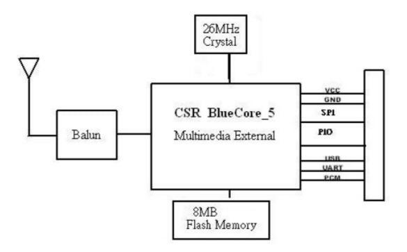
Fig 1.3 SBC05-AT Class2 Module Block Diagram
