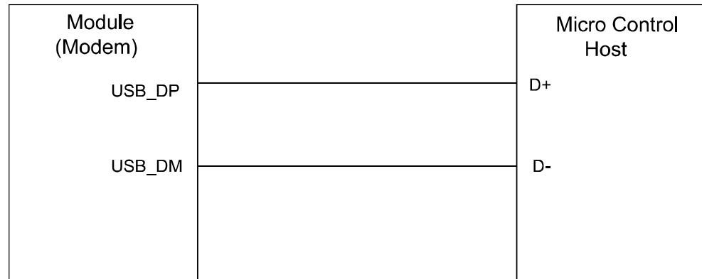
Figure 3-8 Recommended circuit of USB interface
