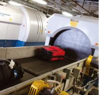
Morpho Detection's CTX 9800 DSi™ represents the latest evolution in CTX™ explosives detection system (EDS) technology. The CTX 9800 DSi introduces a new Data Acquisition System (DAS) that delivers unprecedented high-resolution 3D images. This unique high-resolution imaging engine, called Clarity, represents the culmination of Morpho Detection's years of aviation security experience around the world combined with GE Healthcare's leading-edge imaging technology.
