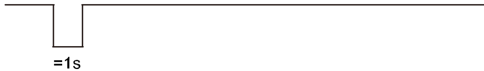
Figure 3-9 The signal through the RING after the MG301 B2B receives an SM
