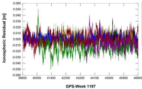
Figure 5: Double differenced ionospheric residual, NO ionosphere, baseline 50km.
