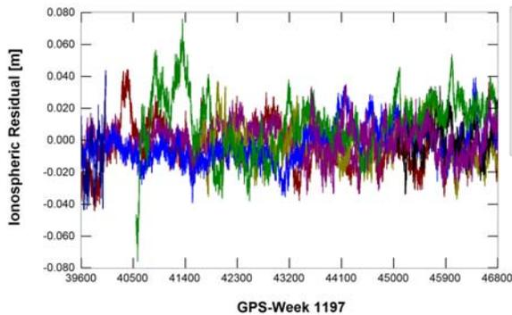
Figure 7: Double differenced ionospheric residual, with ionosphere after application of VRS, baseline 50km.
