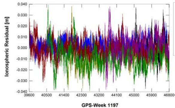
Figure 2: Double differenced ionospheric residual, NO ionosphere, baseline 10km.
