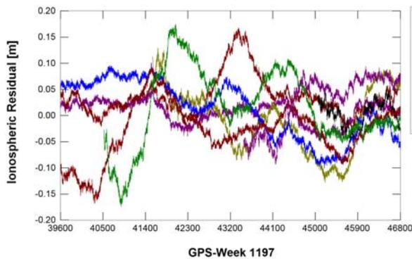
Figure 6: Double differenced ionospheric residual, with ionosphere, baseline 50km.
