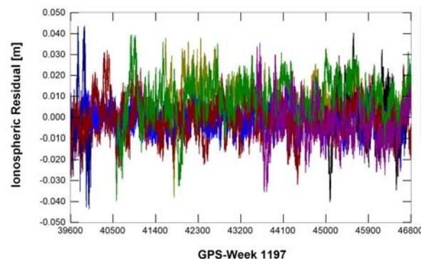
Figure 4: Double differenced ionospheric residual, with ionosphere, after application of VRS, baseline 10km.
