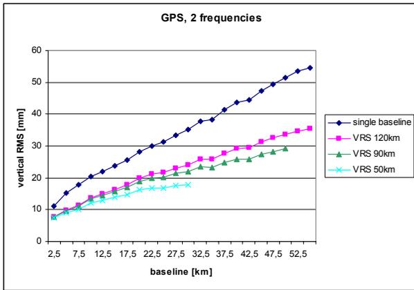
Figure 14: Vertical RMS, GPS, 2 frequencies.
