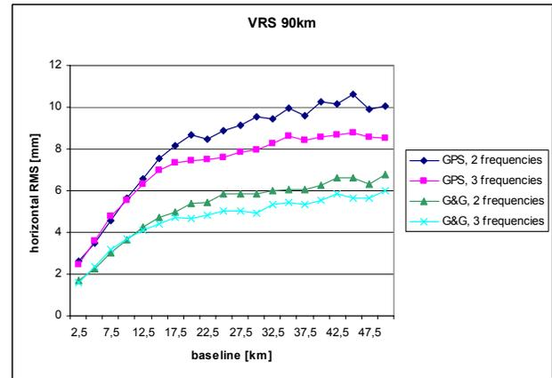
Figure 17: Horizontal RMS, VRS 90km.
