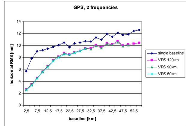
Figure 18: Horizontal RMS, GPS, 2 frequencies.
