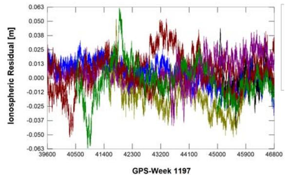
Figure 3: Double differenced ionospheric residual, with ionosphere, baseline 10km.
