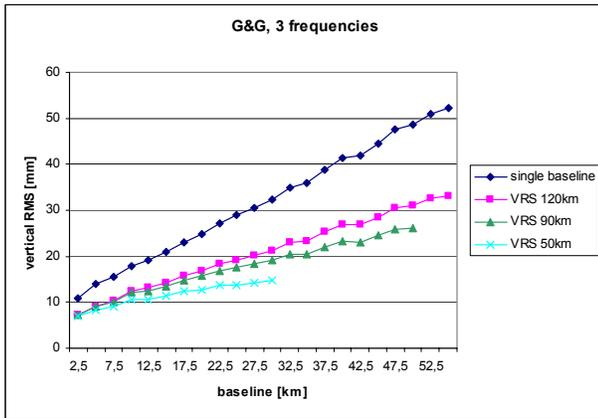
Figure 15: Vertical RMS, GPS, 3 frequencies.
